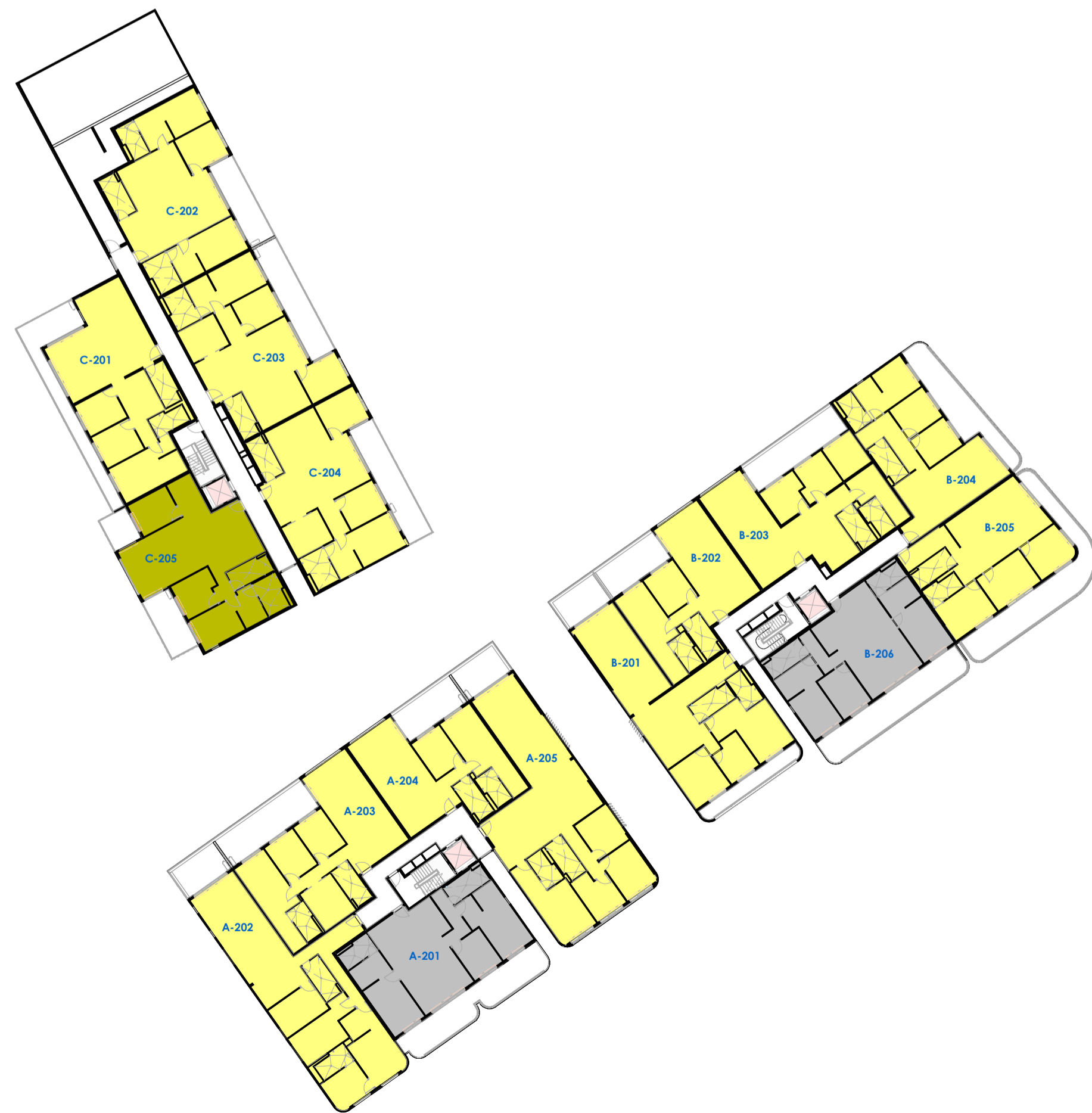
SOLAR ACCESS DIAGRAM - LEVEL 02
