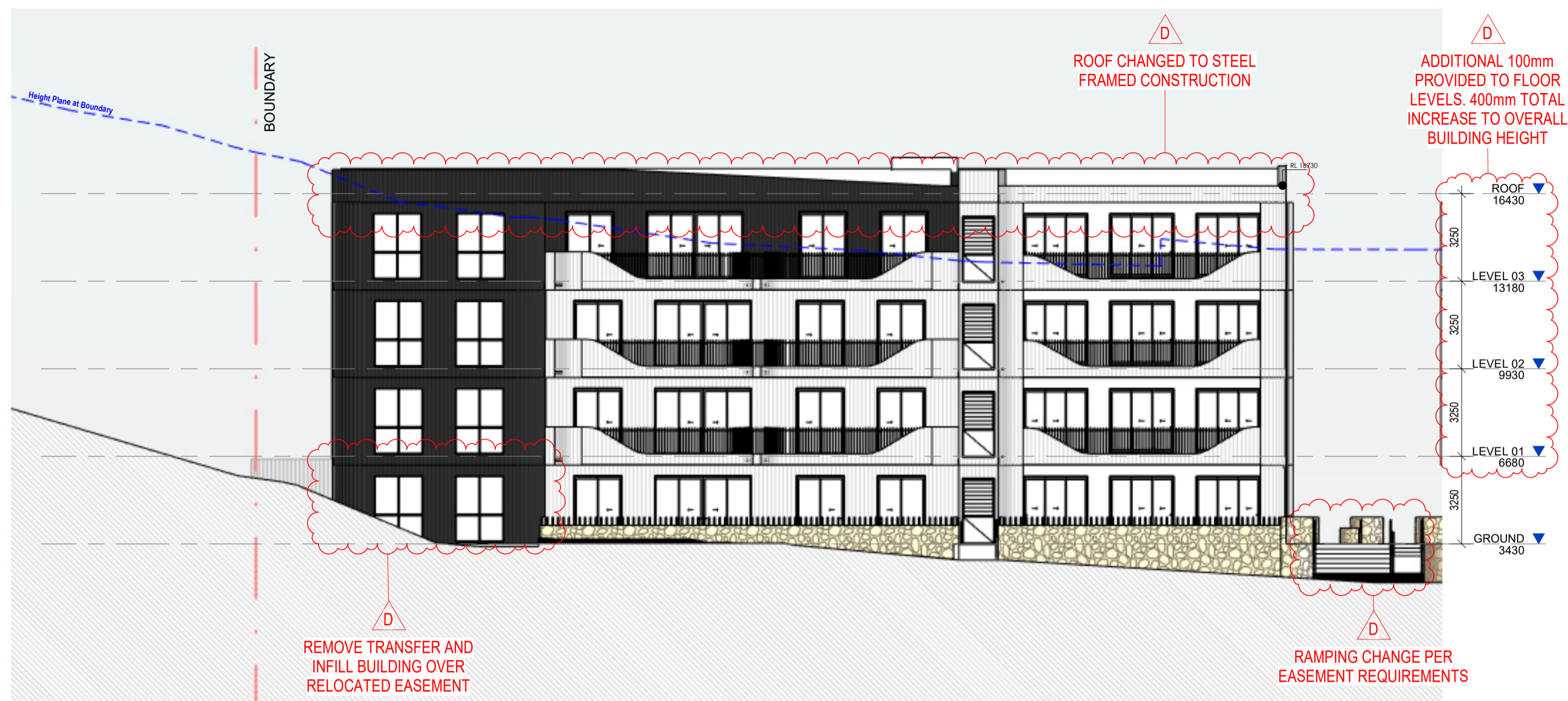
BUILDING A - SOUTH ELEVATION
